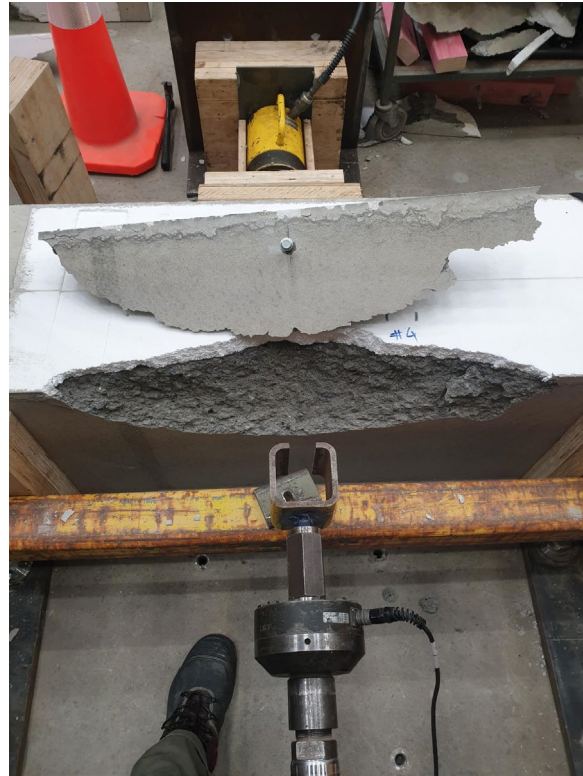
Figure 11. 10 x 150mm HUS4-H Hilti threaded anchor after tension testing.
