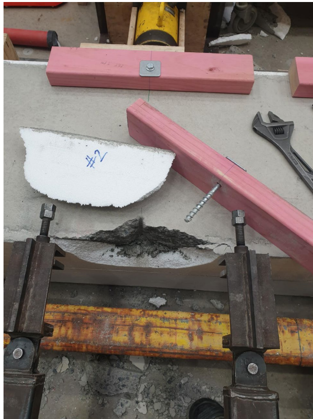
Figure 10. 10 x 150mm HUS4-H Hilti threaded anchor after failure from out of plane testing.
