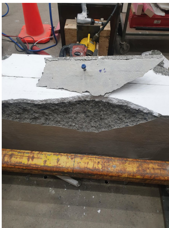
Figure 7. M10 x 140 mm Bowmac Anchor after failure from tension testing.
